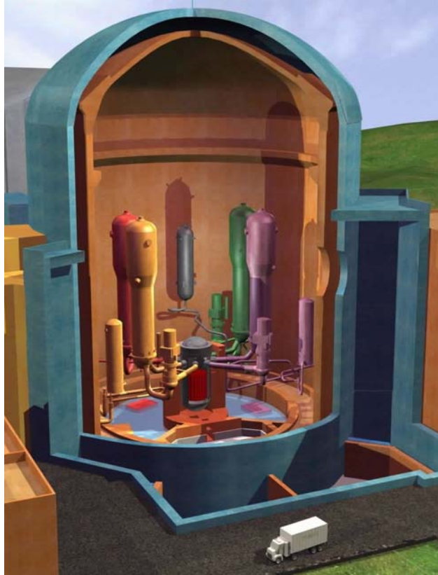
Figure 3: Cutaway View of the U.S. EPR Standard Design
