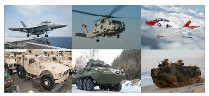
F/A-18F Super Hornet, Two-Seat Model, MH-60R Helicopter, and T-45 Goshawk (top, left to right) Mine Resistant Ambush Protected Vehicle, Light Armored Vehicle, and Assault Amphibious Vehicle (bottom, left to right) Source: U.S. Marine Corps and U.S. Navy.
