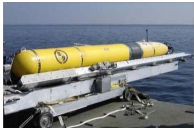
**Unmanned Undersea Vehicle Launch and Recovery Device**
