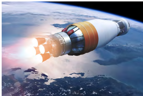
The Exploration Upper Stage is a four-engine in-space stage on the SLS Block 1B and Block 2 rockets, which will be used for Artemis IV and beyond.
