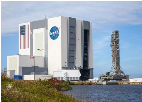
ML-1 rolls back to the Vehicle Assembly Building after integration testing at Launch Pad 39B
