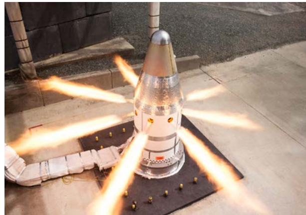
A static hot-fire test of the Orion spacecraft's Launch Abort System Attitude Control Motor
