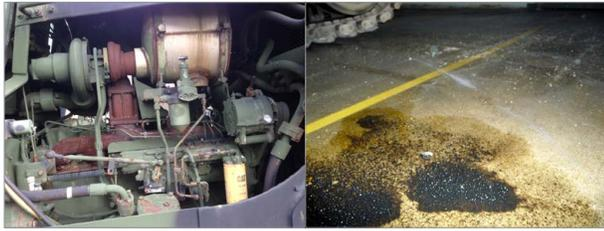
**Photos of Full-Track Tractor with Engine Corrosion (left) and Armored Bridge Vehicle Class III Leak (right)**
