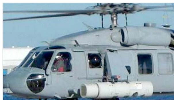
**Airborne Laser Mine Detection System**
