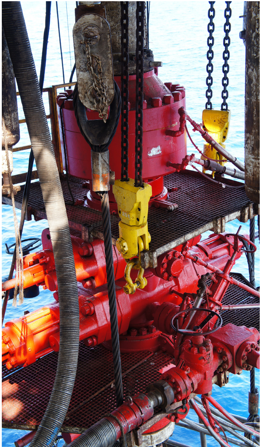
Offshore oil well blowout preventer.
