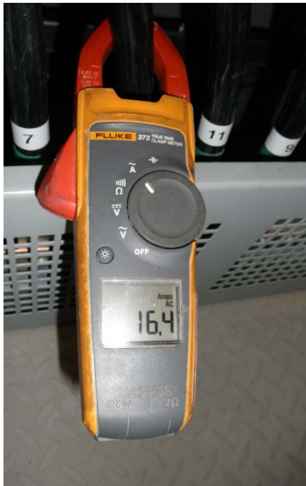
Figure 1: Objectionable Current Reading Taken February 14, 2016 – New Office Annex (NOX) Basement Switchgear Room. (OIG photo)
