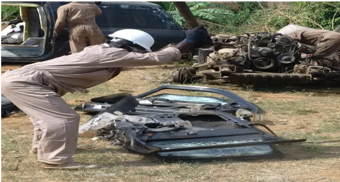
Figure 3. A contractor without proper protective footwear smashing ballistic glass.
