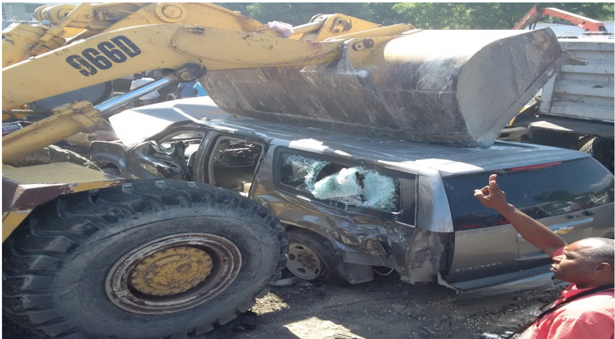
Figure 6. A front-end loader attempting to smash the vehicle while a Department employee who is providing instruction to the contractor stands nearby without personal protective equipment.
