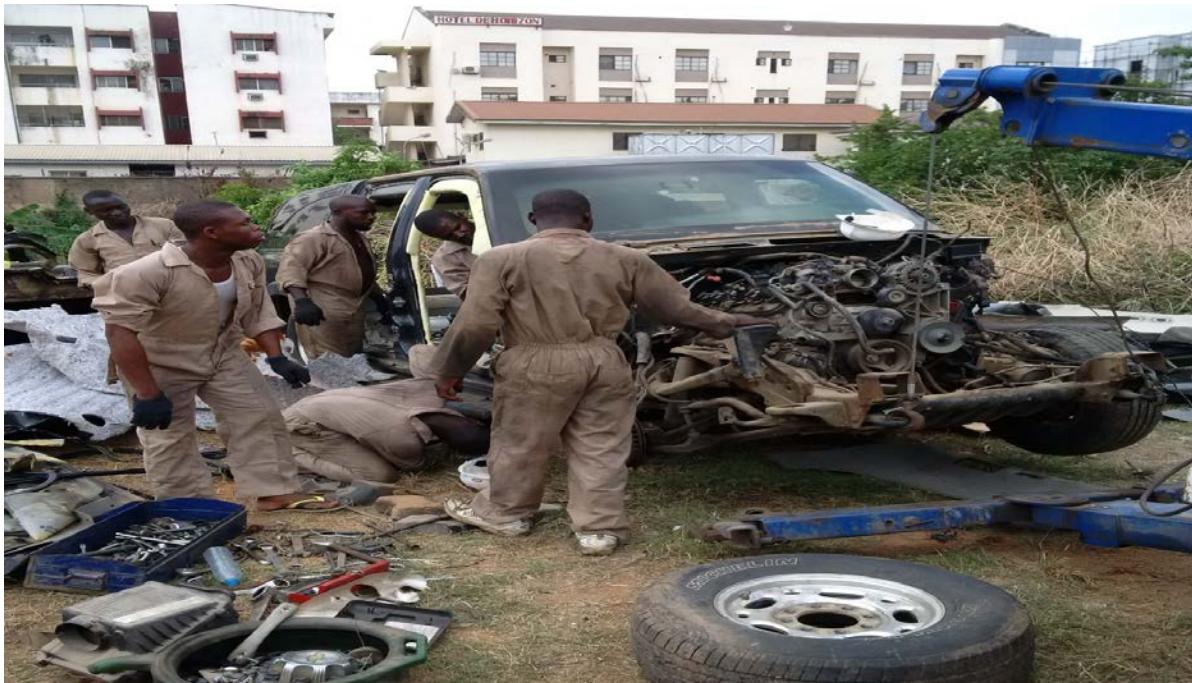
Figure 4. Contractors working in flip flops, without personal protective equipment, and under the vehicle while other men are in the vehicle, which is being suspended by a metal chain from a tow truck.
