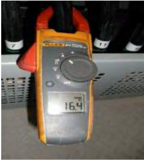
Figure 2: Objectionable Current Reading in NOX Basement Switchgear Room.
