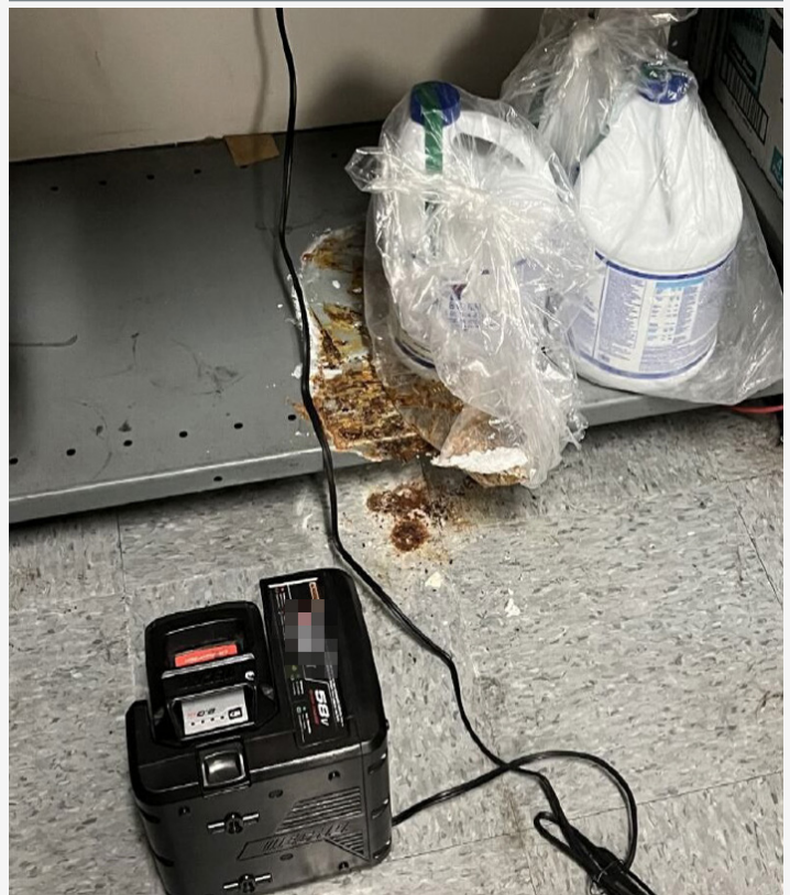
Figure 7. Improper Storage of Cleaning Solution Near Charging Device in Storage Room
