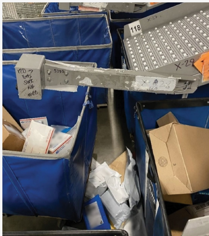
Figure 3. ADUS Operated With an Ineffective Sweeper
