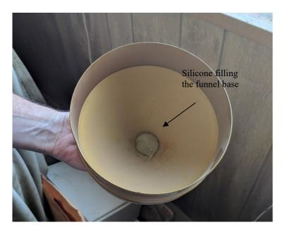
**Figure 1.** This rain gauge was tampered with by filling the funnel with silicone to prevent water from entering the gauge to be measured. OIG photo.
