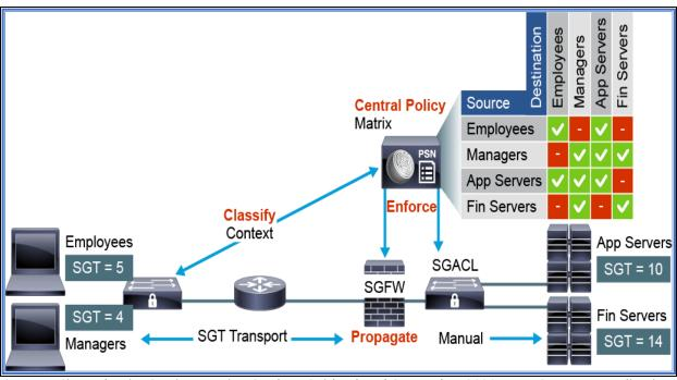
Figure 2: TrustSec Classification, Propagation, and Enforcement of the Security Group Tags
