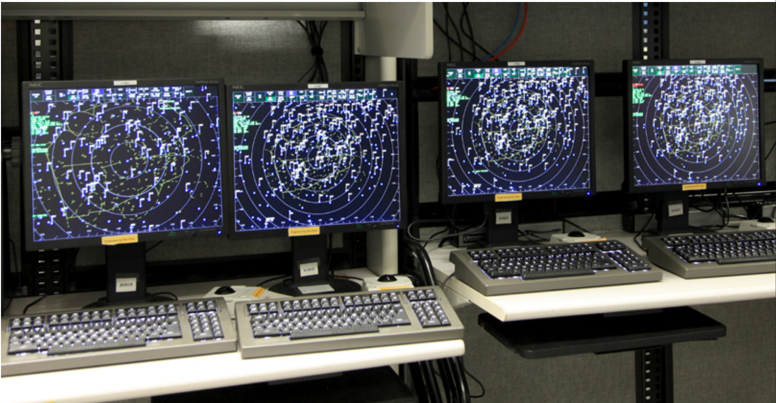
STARS monitors. STARS, a foundational system for NextGen, stands for Standard Terminal Automation Replacement System. Photo: FAA
