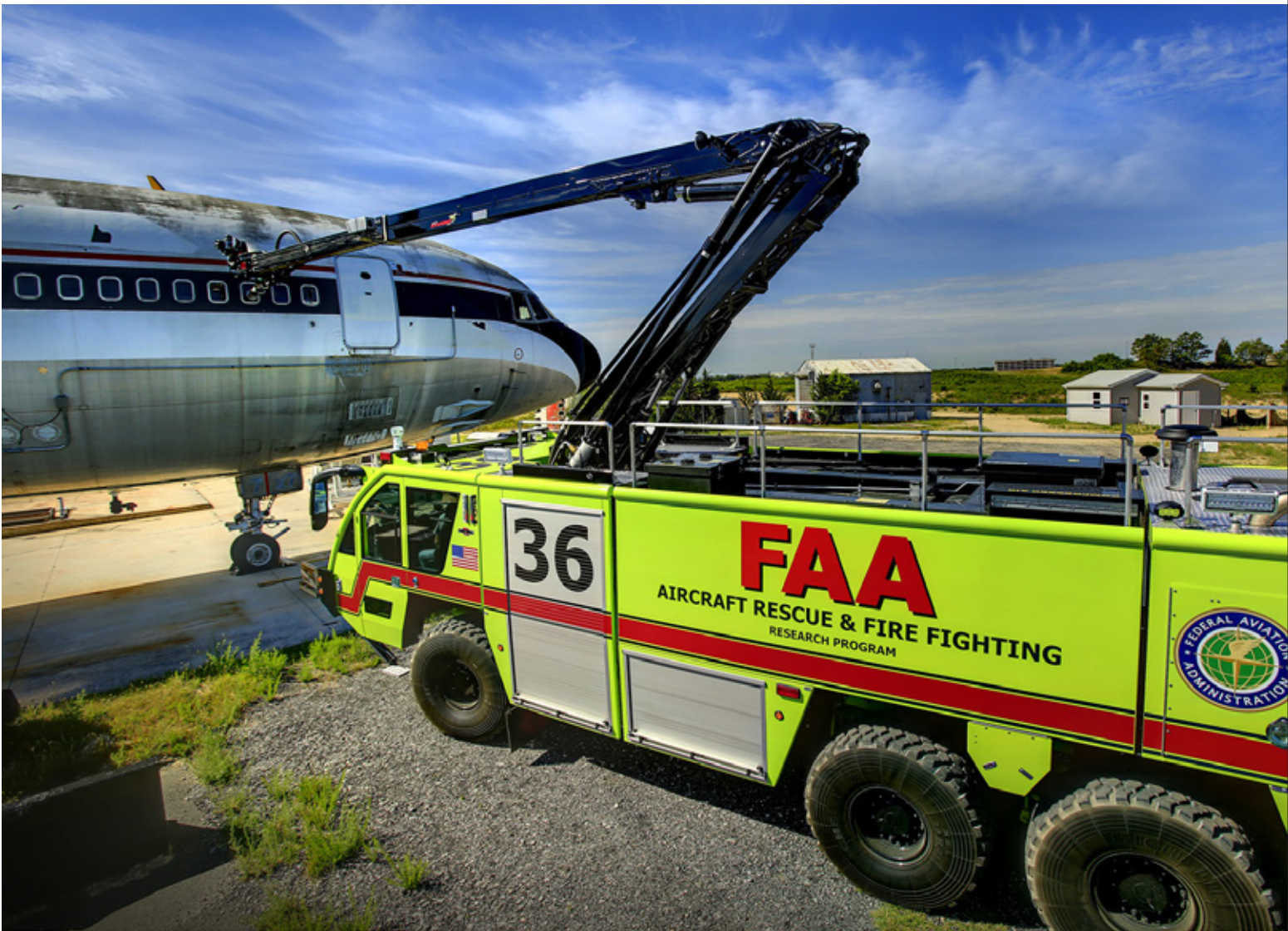
The operator of the FAA's Rosenbauer Panther Aircraft Rescue and Fire Fighting research vehicle positions the piercing nozzle of the high-reach extendable turret at the window of the L-1011 test aircraft. Research conducted with this vehicle is intended to develop improved technologies in aviation fire fighting and increase post-crash survivability of passengers in future aircraft accidents. William J. Hughes Technical Center.
