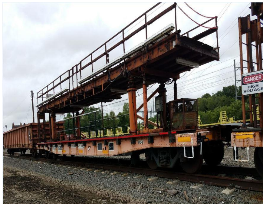
Figure 3. An Example of a Catenary Tower Car the Department Could Not Account For
