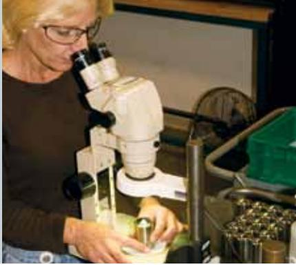
**After completing the turning and polishing process, Pamela Allendorf inspects blank dies before they become production dies.**
