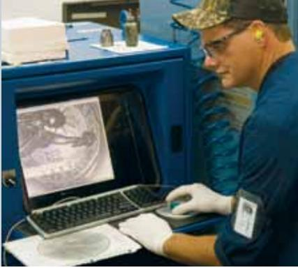
**Christopher Hyde operates a turning lathe to machine the outside diameter of a dollar coin reverse die. He can watch the machining process on-screen.**
