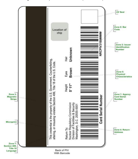
Figure 2: Sample NRC PIV Card (Back View)
