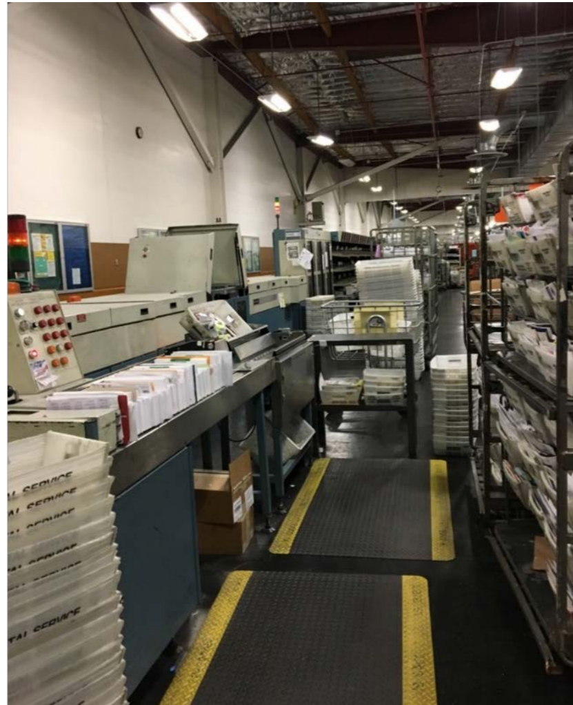
Figure 2. Idle Machine Loaded with PARS Mail and Awaiting Processing
