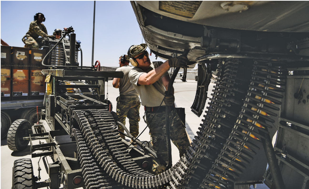
U.S. Air Force weapon loaders load a seven-barrel autocannon on an A-10 Thunderbolt II at Kandahar Airfield. (U.S. Air Force photo)
