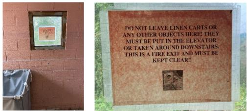
**Photograph 4 (left):** This cart obstructed building exit from a fire exit path. There is also a sign telling workers to keep the area free of carts. **Photograph 5 (right):** This is a close-up of the sign in Photograph 4. The sign reads, "Do not leave linen carts or any other objects here! They must be put in the elevator or taken around downstairs. This is a fire exit and must be kept clear!!"
