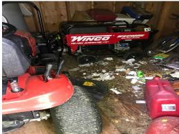
**Photograph 20:** A generator was stored in a wooden shed with full gas canisters. An animal was nesting in the shed.
