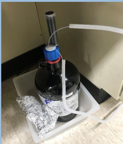
An improper waste container found during an EPA lab inspection. (EPA image)
