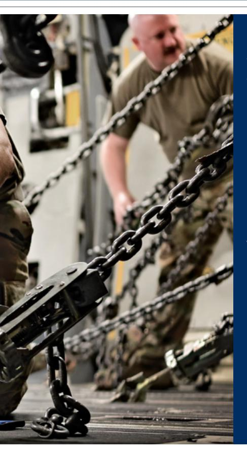
A U.S. Air Force C-17A Globemaster III aircraft loadmaster measures the restraints on a U.S. Army M1A2 Abrams Main Battle Tank at Ali Al-Salem Air Base, Kuwait. (U.S. Air Force
