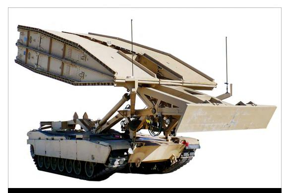
Figure 3. The Joint Assault Bridge Source: The U.S. Army Acquisition Support Center.
