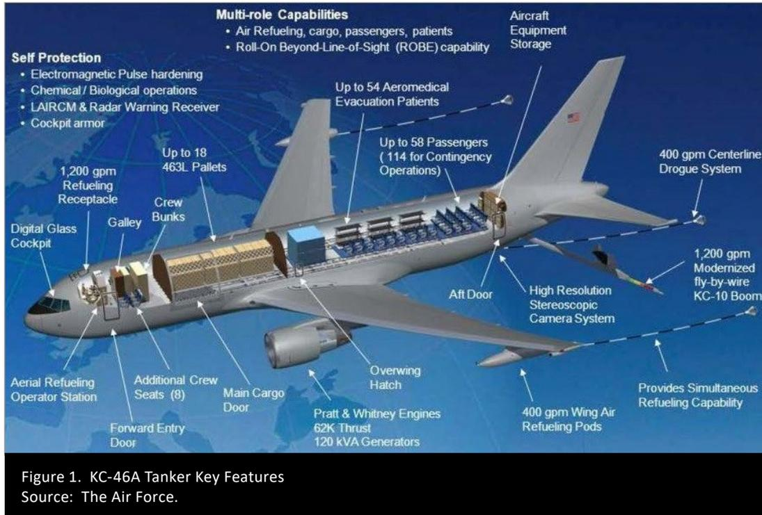
Figure 1. KC-46A Tanker Key Features
