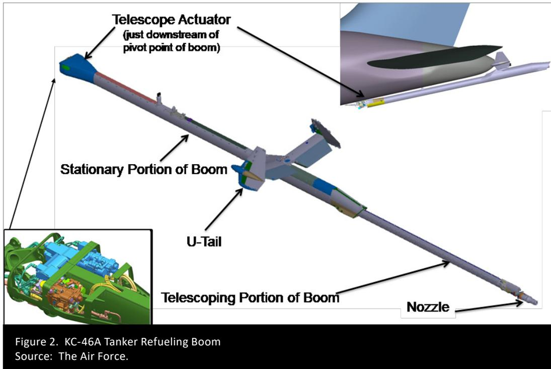
The refueling boom is the component of the aerial refueling system that transfers fuel from the KC-46A tanker to the receiver aircraft. A receiver aircraft is any DoD or allied aircraft capable of being aerially refueled. During aerial refueling, an operator on the KC-46A tanker extends the refueling boom into a receptacle on the receiving aircraft to transfer fuel. The goal of aerial refueling is to extend the range or time a receiver aircraft can remain in the air.
