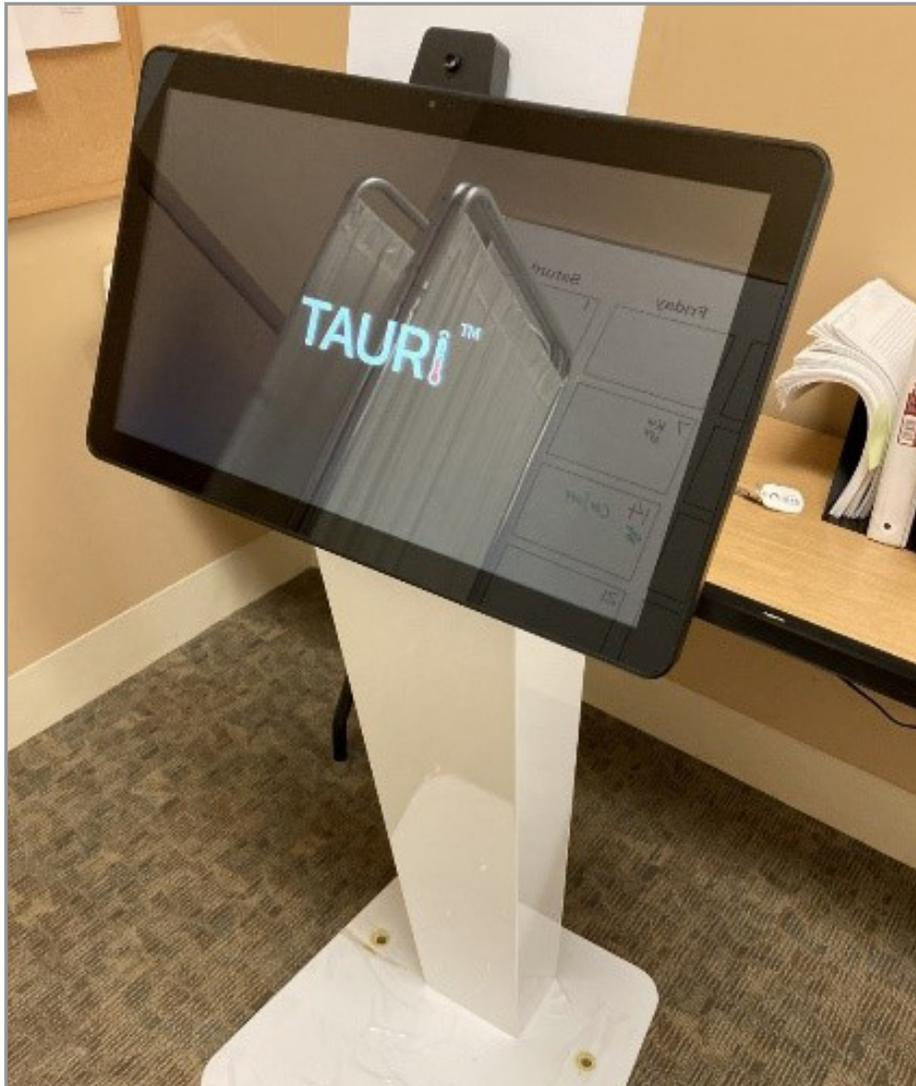
Figure 3. Temperature-Measuring Kiosk Located at the Entrance of the AFRH-W Facility
