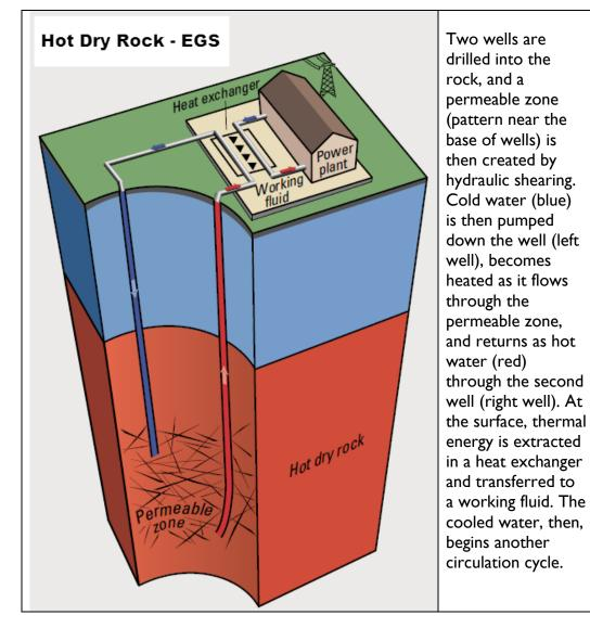
Figure 2. Hot, dry rock EGS. Source: USGS<sup>2</sup>
