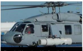
Figure 4. Airborne Laser Mine Detection System Source: PEO LCS.
