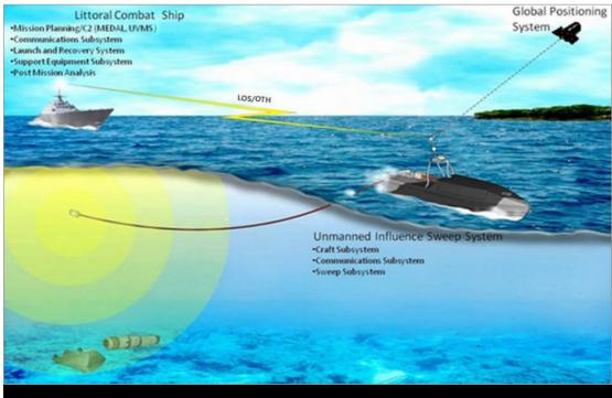
Figure 6. Unmanned Influence Sweep System Simplified Operational Concept Source: PMS 406.
