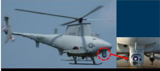
Figure 5. Coastal Battlefield Reconnaissance and Analysis Block I Payload on MQ-8B VTUAV Source: PMS 420.
