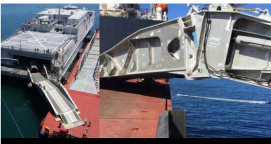
Figure 2. EPF Stern Ramp and Mobile Landing Platform Used for At-Sea Transfers. Source: COMOPTEVFOR FOT&E Report.
