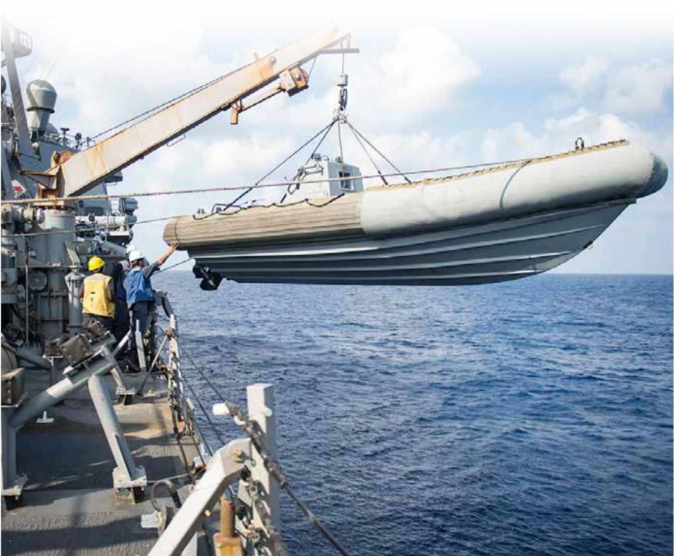
Sailors prepare to launch a rigid-hull inflatable boat from the boat deck. (U.S. Navy photo by Petty Officer 3rd Class Bill Dodge/Released)
