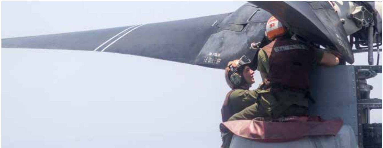
U.S. Marines prepare to dismount a rotor of an MV-22 Osprey. Photo by Cpl Kyle N. Runnels.
