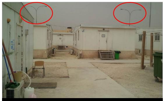
Figure 4. Two nonoperational lights Source: DoD OIG
