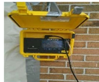
Figure 4 – Asbestos meter and containment 310 Highland Ave.
