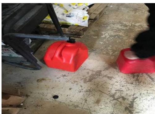
Photograph 10 (left): Unsecured gasoline cans not stored in a flammables storage cabinet. Photograph 11 (right): Oxygen storage room lacking a posted “NO SMOKING” sign or symbol.
