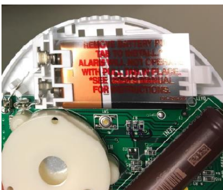
Photograph 7: Carbon monoxide detector installed without removing the factory-provided battery tab.
