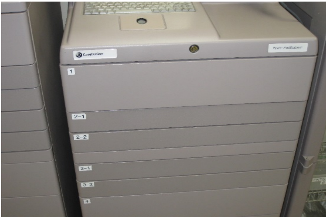
Photograph 2: Secured compartments of the Pyxis system that keep Scheduled drugs from being dispensed inappropriately at Burdick Memorial.
