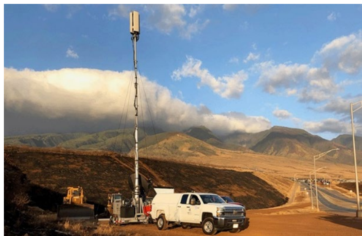
Figure 6. Mobile FirstNet cell sites like this one connect via satellite to provide network coverage.
