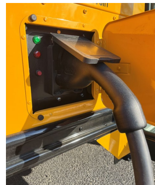
An electric school bus being charged. (EPA OIG image)
