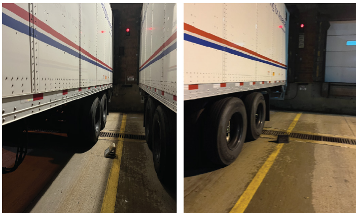
Figure 2. Trailers Without Wheel Chocks
