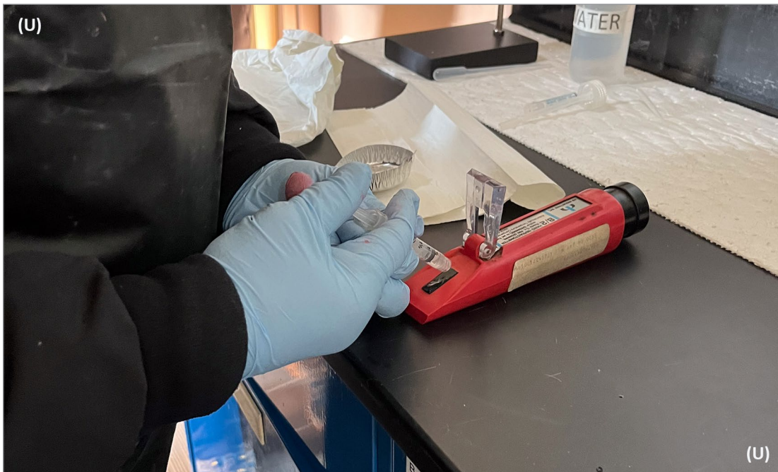
(U) Figure 9. FSII Test Conducted on January 17, 2025, at Daegu DFSP, South Korea (U) Source: The DoD OIG.
