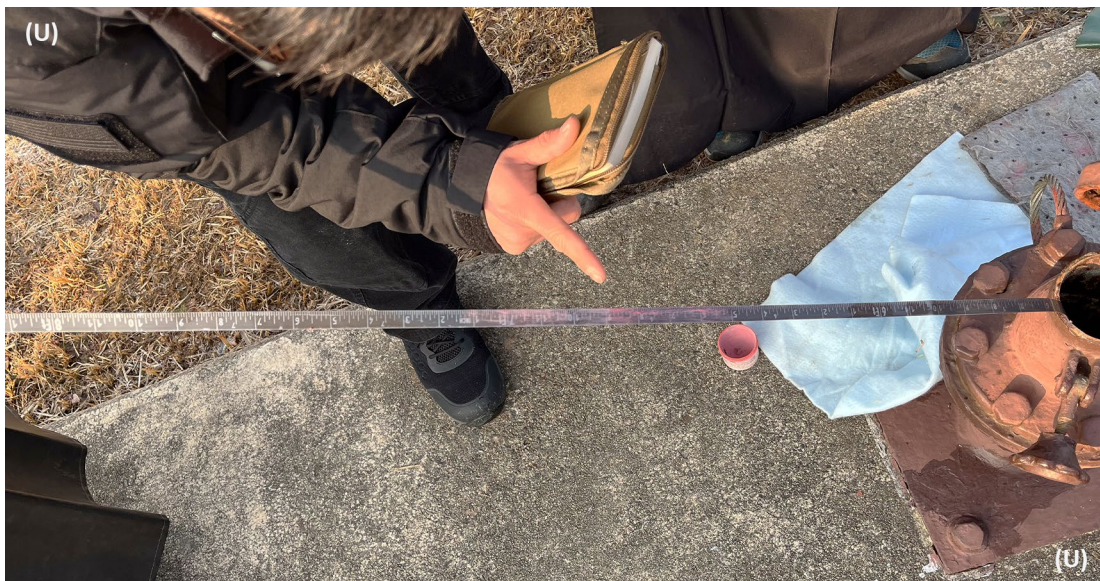
(U) Figure 7. Manual Gauging During ATG Verification (U) Source: The DoD OIG.
