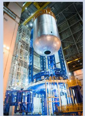
The Vertical Assembly Center is the world's largest spacecraft welding tool. It was specifically designed to build the Space Launch System core stage. Located at the Michoud Assembly Facility in New Orleans, Louisiana, the Vertical Assembly Center is governmentheld property used by the Space Launch System contractor on-site. Pictured here, a liquid oxygen tank confidence article completes final welding to verify weld procedures are working as planned.
