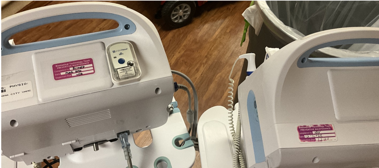
Figure C.1. Similar pieces of equipment with inconsistent preventive maintenance inspection documentation. Source: Photo taken by OIG inspector.
