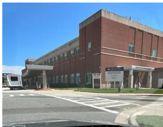
Figure C.3. Photo of main (left) and Emergency Department (right) entrances with example of a crosswalk with missing detectable warning surfaces (features to alert visually impaired pedestrians of a hazard in the line of travel).
