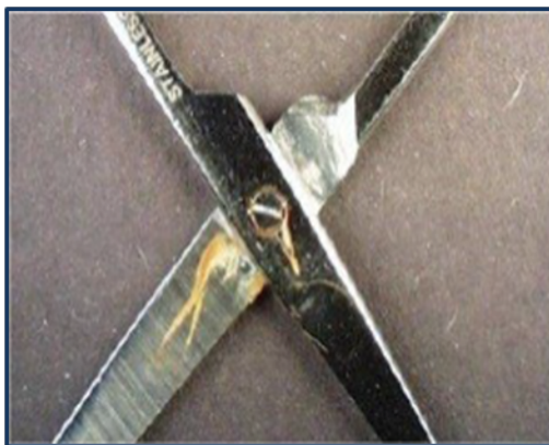
Figure 1: Example of nonconformities on surgical instruments including corrosion, pitting, rusting, and stress cracking.
