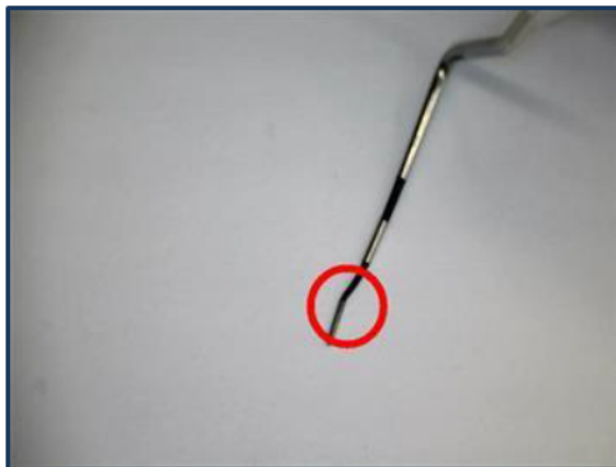
Figure 3. Dental pick from restorative tray 45 prior to undergoing repair.
