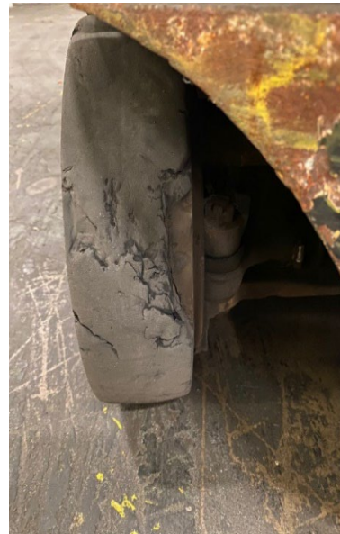
Figure 6. A portion of Tire Missing from A Powered Industrial Truck
