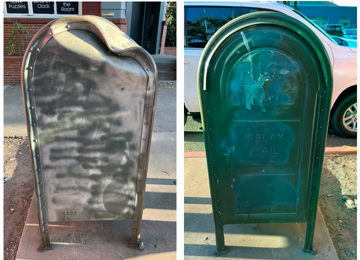
Figure 9. Sacramento, CA, Green Relay Box With Dent and Corrosion
