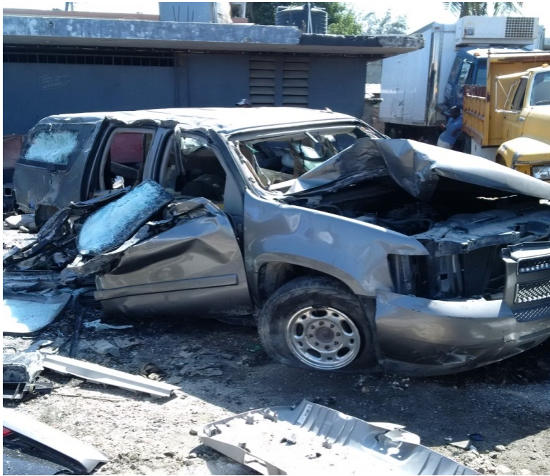
Figure 11: End result of armored vehicle disposal in Port-au-Prince, Haiti, showing intact armor.
