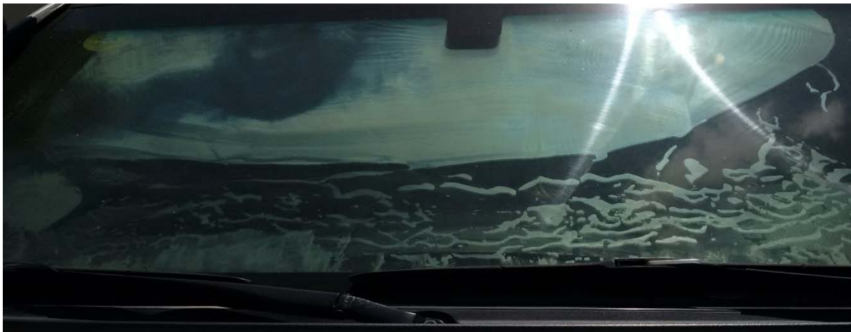
Figure 7: Armored vehicle at Embassy Port-au-Prince with significant ballistic glass delamination, including bubbling. Source: OIG photograph taken at Embassy Port-au-Prince on February 23, 2016.
