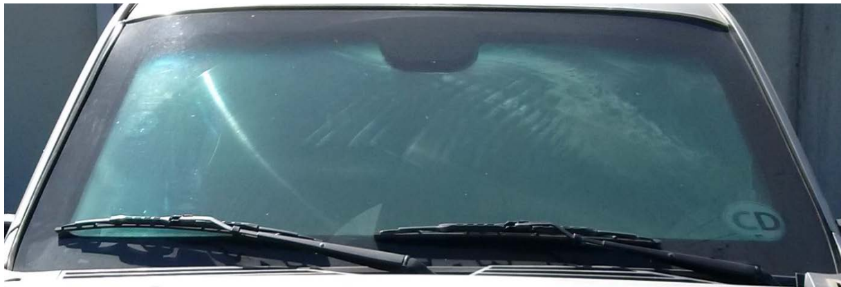
Figure 8: Armored vehicle at Embassy Port-au-Prince with significant ballistic glass delamination, including ghosting. Source: OIG photograph taken at Embassy Port-au-Prince on February 23, 2016.
