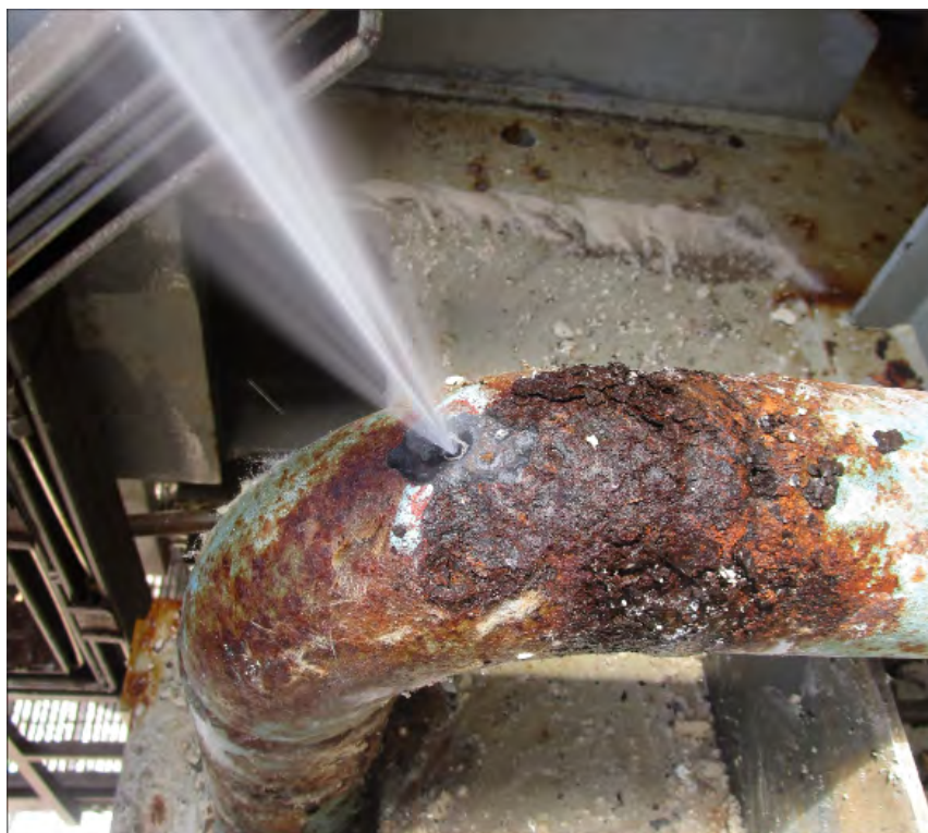
Figure 1: AFW Leak at DCNPP
