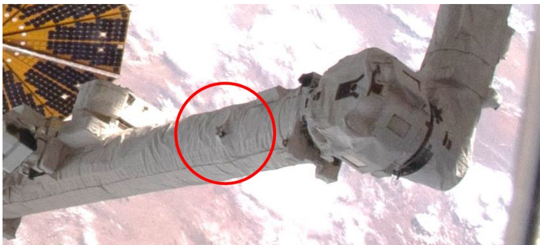
Figure 4: Canadarm2 Orbital Debris Strike, May 2021
