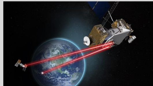
Conceptual Image of LCRD Relaying Data Between the International Space Station and the Ground
