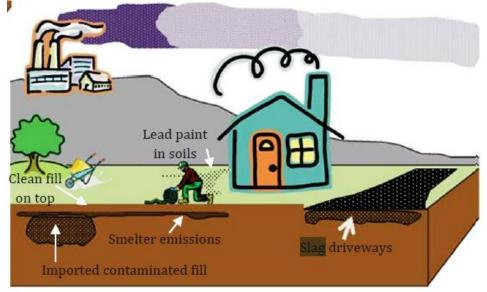
Figure 2: EPA's conceptual site model for the Anaconda site, 2013 revision
